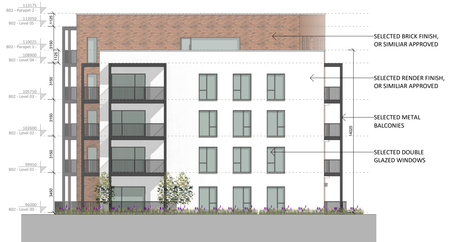
② Block 02 - South Elevation 1 : 200
